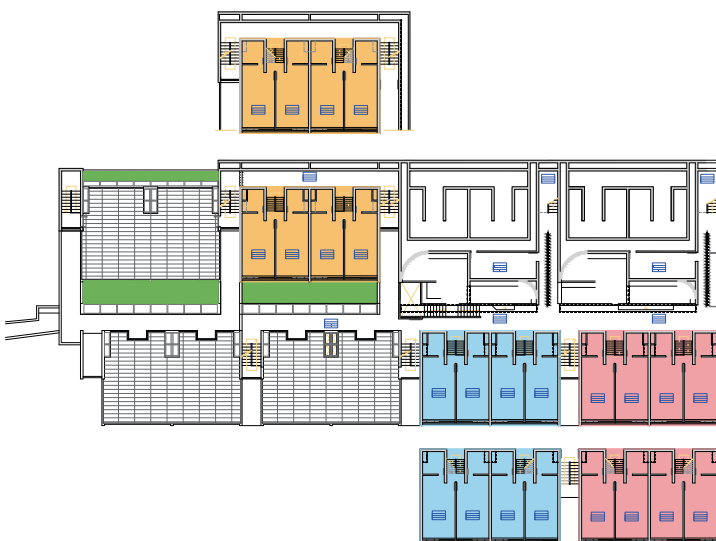
Each part of the complex (blocks, rooms, com-mon spaces, internal and external paths, external spaces) has been identified through an alphanumeric code, reported on plans, which contains also the dimensions and the use of each room. For each room, it will therefore possible to insert the data on the state of conservation, to keep track of the maintenance works realised and of the costs and to control the use and the specific issues of each space.
